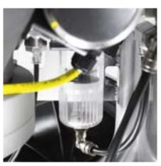
With integrated oil and water separator
